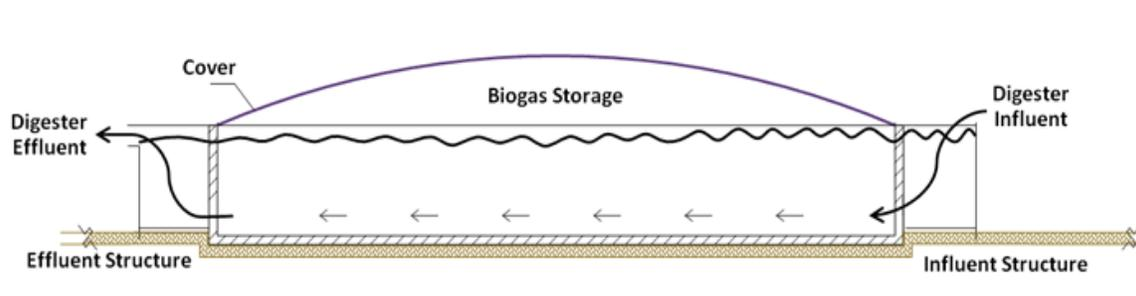
**Figure 29. Diagram of a Plug Flow Digester**
